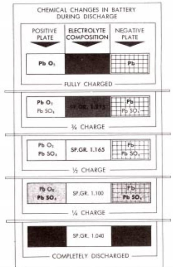
Chemical changes in battery during discharge.
