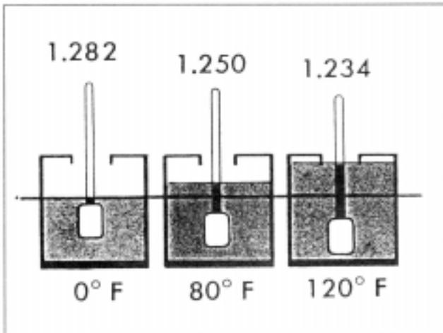
Compensation for specific gravity variations caused by temperature changes.
