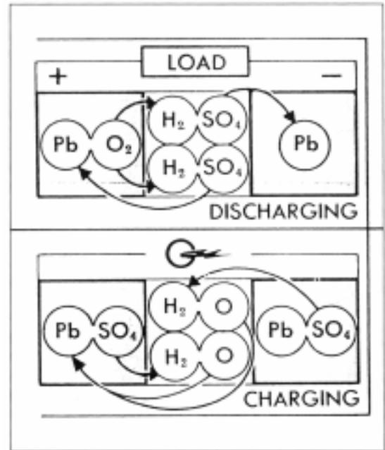
Chemical reactions occurring in the battery cell during charge are basically the reverse of those which occur during discharge.
