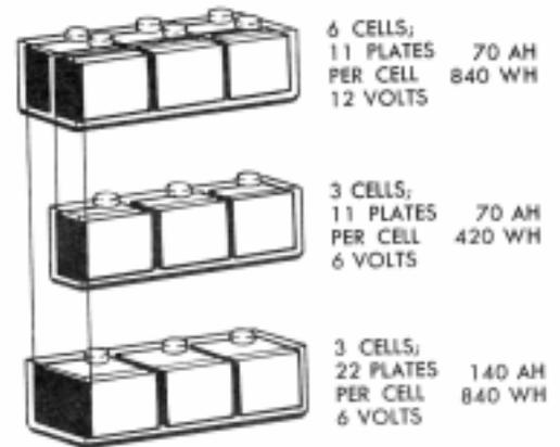
A comparison of ampere-hour capacities of 6- and 12-volt batteries.
